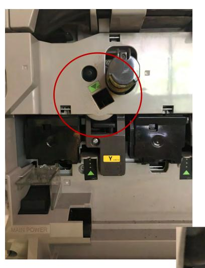
Step 4: Locate green sticker with black triangle. Insert green cleaning wand, roller side facing up, into the hole below the green sticker. (Black triangle on the end of the green wand will be facing upright). Carefully push green wand back as far as it will go (It will no go back the entire length of the wand). Run the cleaner front to back a few times. Repeat for each color- (Y, M, C, B)
