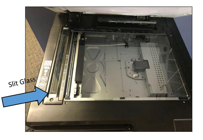
Using a cloth/paper towel and Windex or denatured alcohol, clean both the copy glass and the slit glass. Lines on copies and scans could be caused by marks or even a hair on the glass.
