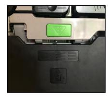
Press in on bright green button to release waste container from locked position.
