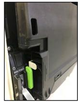
Press in green tabs on both ends of the waste container to release.
