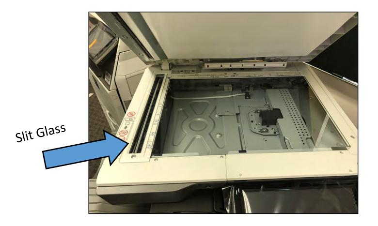
Using a cloth/paper towel and Windex or denatured alcohol, clean both the copy glass and the slit glass. Lines on copies and scans could be caused by small marks or even a hair on the glass.
