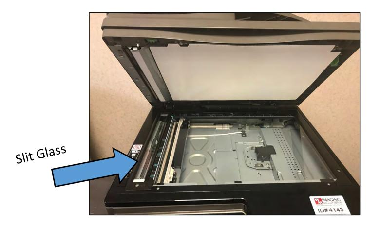
Using a cloth/paper towel and Windex or denatured alcohol, clean both the copy glass and the slit glass. Lines on copies and scans could be caused by marks or even a hair on the glass.
