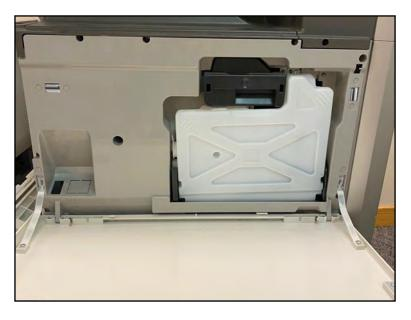
Gently pull the end of the cleaning rod out of the machine, towards you, as far as it will go. It will not come out of the machine completely. Push the rod back into the machine—Repeat a few times.
