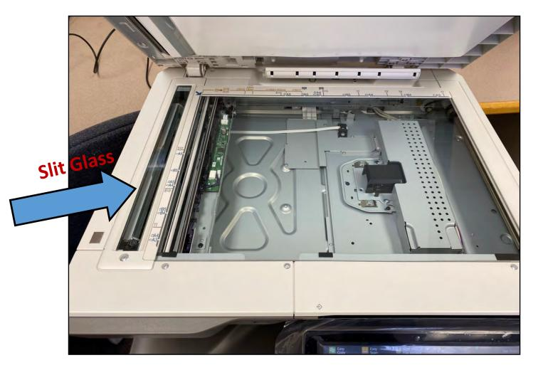
Using a cloth/paper towel and Windex or denatured alcohol, clean both the copy glass and the slit glass. Lines on copies and scans could be caused by marks or even a hair on the glass.
