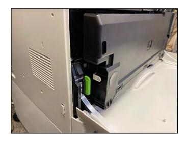
Press in on bright green buttons, located on both ends of the waste container, to release container from locked position.
