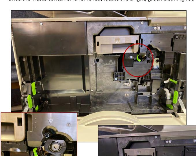
Gently pull the end of the cleaning rod out of the machine, towards you, as far as it will go. It will not come out of the machine completely. Push the rod back into the machine—
